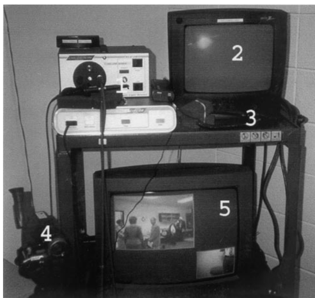
Fig 3. The numbers in the photograph are as follows: 1, endoscope; 2, endoscope monitor; 3, electronic stethoscope; 4, video camera; 5, TV.
